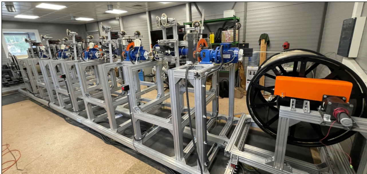
Figure 23. High-current HTS cable winding machine.
